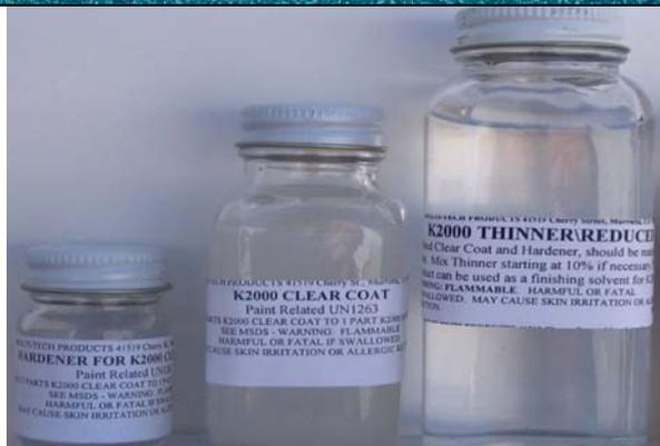
1) Pour an ample amount of K2000 topcoat into a mixing cup or airbrush bottle. Add the hardener in the ratio of 1 part hardener to 3 parts topcoat.
