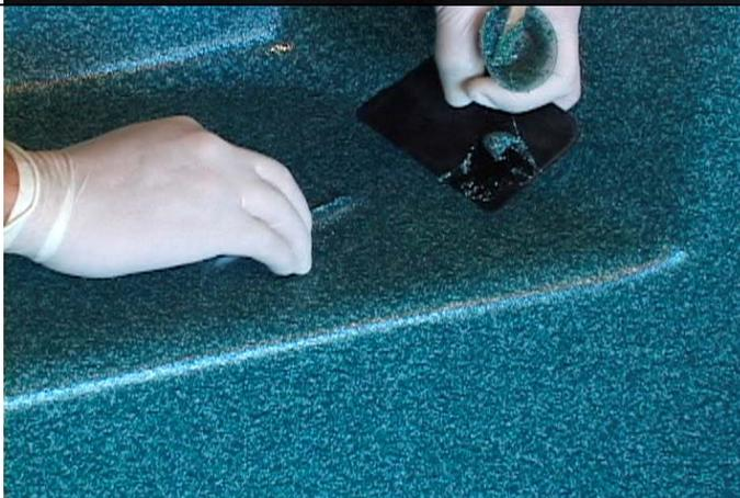
4) Allow it to cure for about ½ hour. The heat gun can be used to accelerate. Direct heat to the immediate surrounding area, and not directly on the filler.
